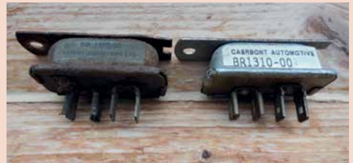
Another view of the BRI310/00's. The one on the right is a modern diode controlled unit
