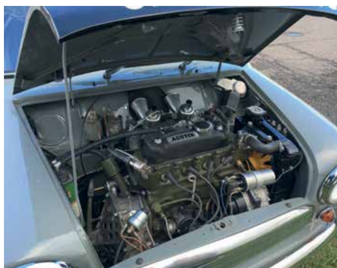
The bonnet's cross frame has been reduced to clear the rocker cover, note no servo
