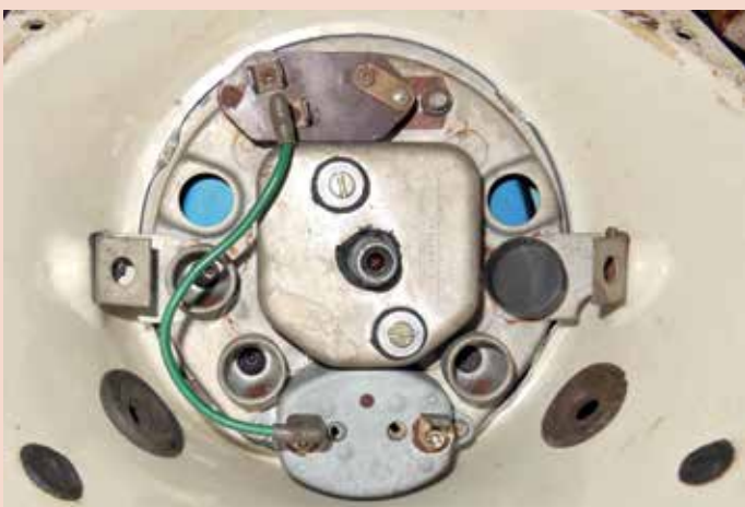
The rear of an SN4417 speedometer. The voltage regulator sits where the top bulb holder was located
