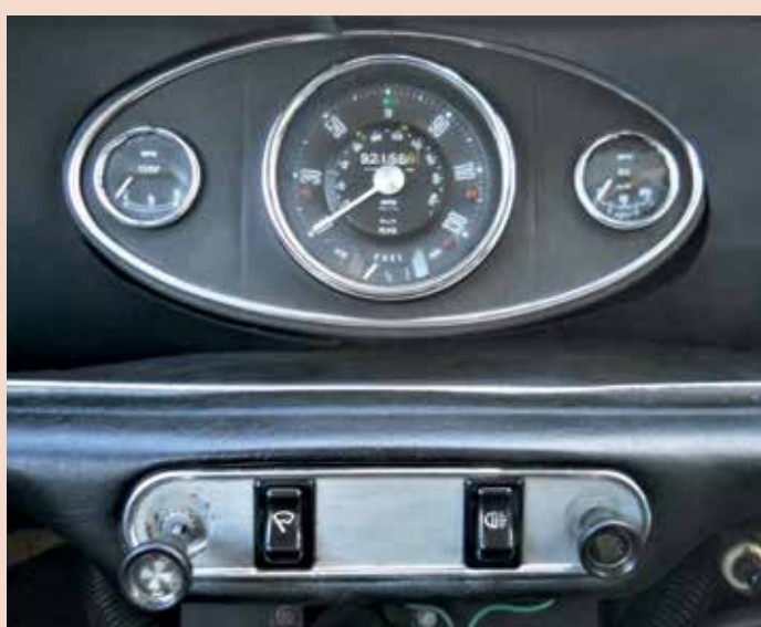
Final spec was just rocker switches and plain panel between the switches
