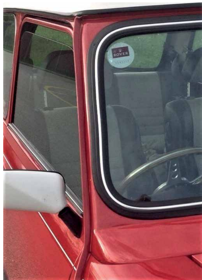
Spot the difference I: The wider front windscreen weatherstrip introduced in early 1993
