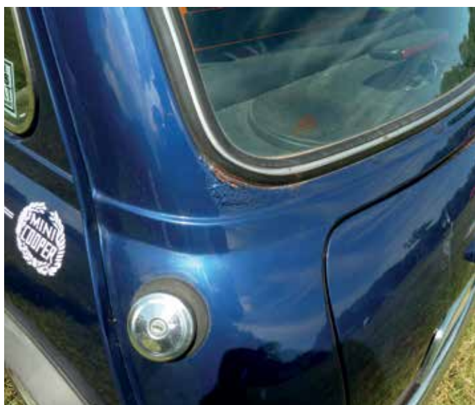
Many corrosion breakouts around the rear windscreen have been attributed to the overzealous use of the production line trimmer's Stanley knife
