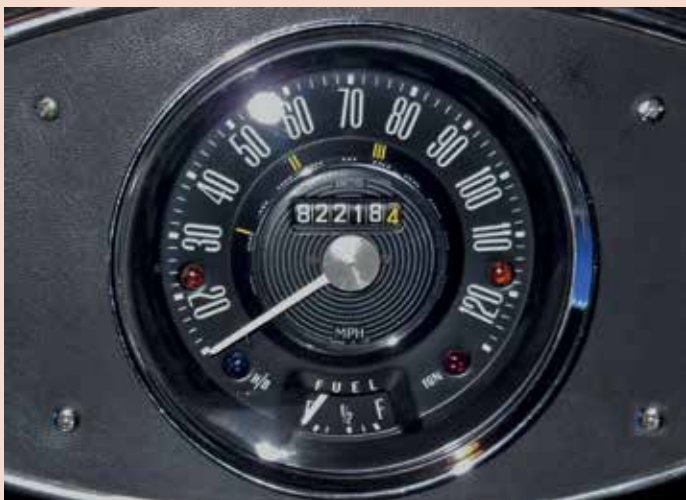
4417/18 speedometer. An orange jewel either side, 70mph at the top and calibration continues to 130mph
