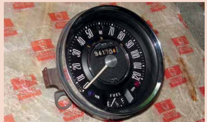
4479/32 speedometer. Blank top 'jewel', 60mph at the top and calibrated to 120mph dead. Early fuel gauge easily distinguished from the later type by the thin needle
