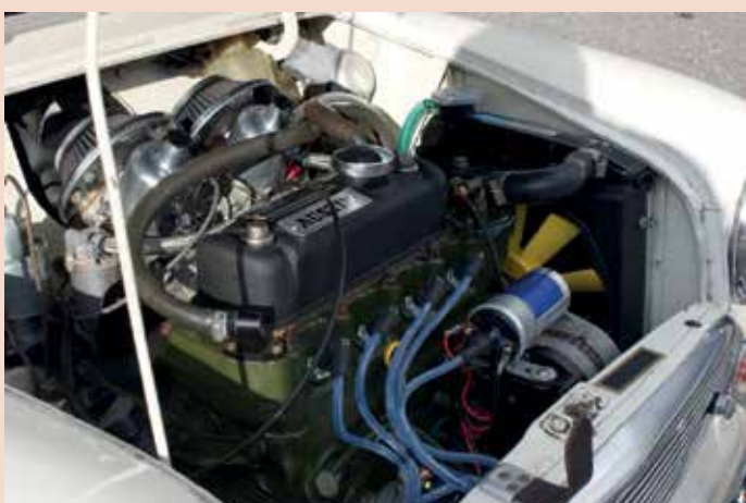
A very neat and tidy engine bay containing a 1293cc motor. The space on the left of the picture is soon to be filled with a servo which will complete the braking upgrade
