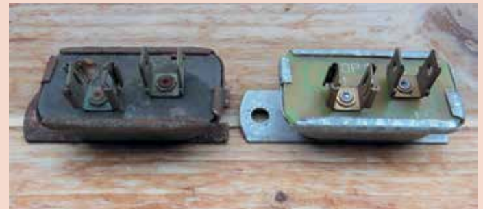
A pair of BRI310/00 stabilisers – note the 'I' female terminal connections
