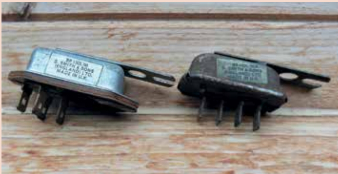
Same part number, different designs. Both have two male dual blade terminals
