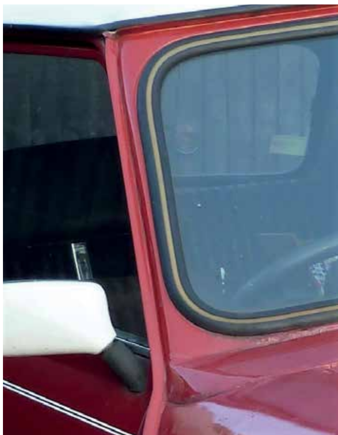
Spot the difference 2: The earlier type of weatherstrip. Note how it neatly fits into the recess to form a good seal
